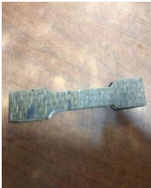
Fig.5 Specimen for tensile test
