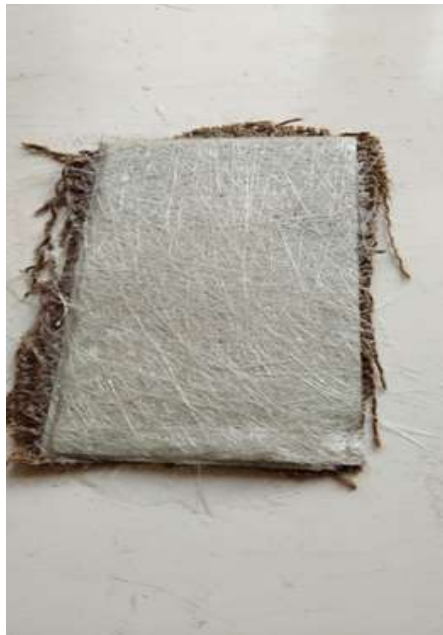
Fig 3. Jute placed on glass fiber sheet
